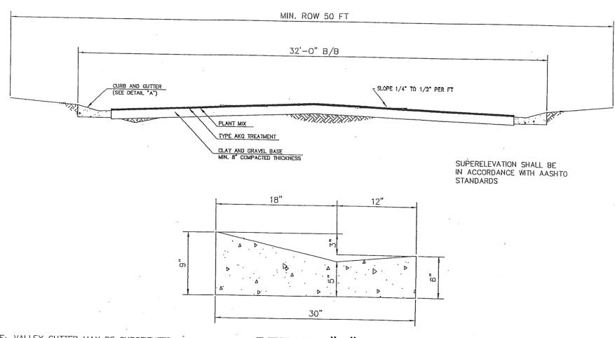
NOTE: VALLEY GUTTER MAY BE SUBSTITUTED FOR COMBINATION CURB AND GUTTER. PAVEMENT WIDTH SHALL NOT BE DIMINISHED.
